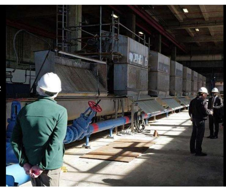
Bar screens are high-wear devices and require frequent maintenance and rebuilding. Here is one of the screens being rebuilt. It has been removed for access and you can see the notches that hold the bars.
